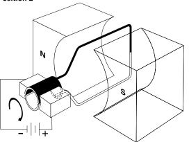
As the conductor continues to rotate from position 2 to position 3 current flows away from the commutator in the white half and toward the commutator in the black half. Current has reversed direction in the conductor. This is known as commutation.
