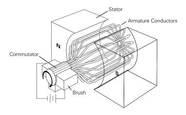
A DC motor rotates as a result of two magnetic fields interacting with each other. The first field is the main field that exists in the stator windings. The second field exists in the armature. Whenever current flows through a conductor a magnetic field is generated around the conductor.
