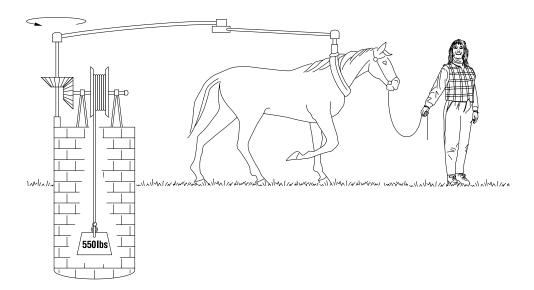
The following formula can be used to calculate horsepower when torque (lb-ft) and speed (RPM) are known. It can be seen from the formula that an increase of torque, speed, or both will cause a corresponding increase in horsepower.
